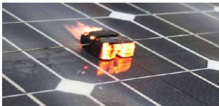
Building Standard , Brand Combustion Test
